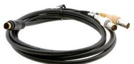
Kramer's s-Video (Y/C) breakout cable is constructed of dual mini coax cables with a male s-Video (4-pin) connector on one end and 2 BNCs on the other. They are used for converting an s-Video signal from the typical 4-pin format to higher quality dual BNC format preferred for long cable runs
